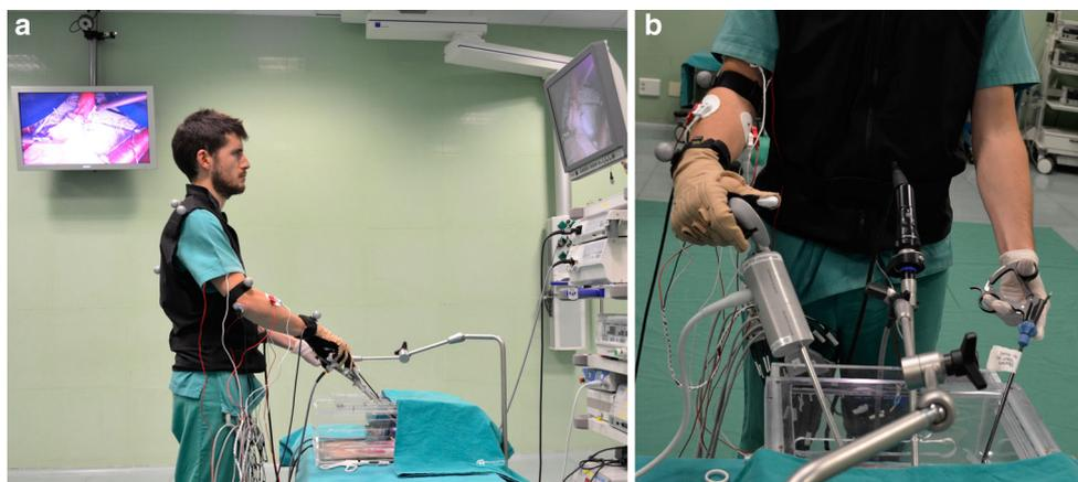
**Fig. 1** Experimental setup for the study. Tasks are performed using both the conventional (a) and robotic (b) needle holders
