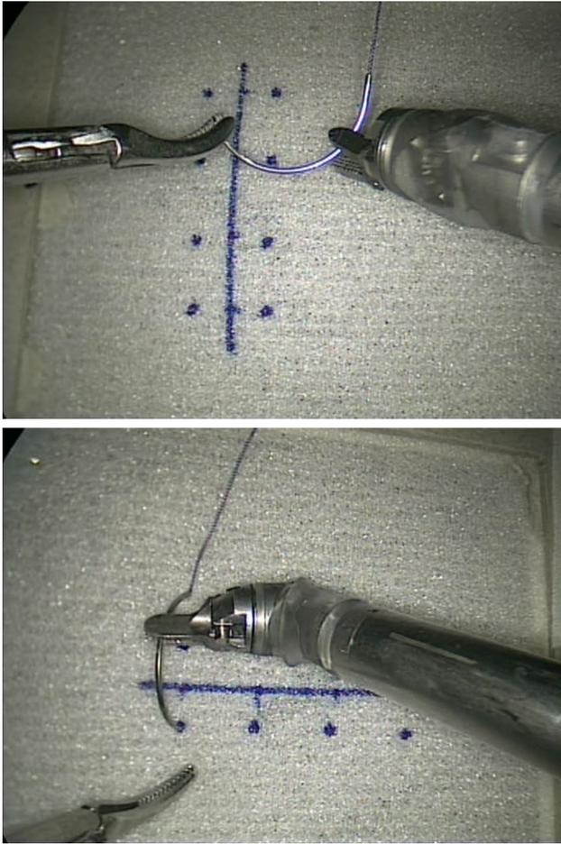
**Fig. 2** Precision task performed using the robotic needle holder. The stitches are carried out following horizontal (*top*) and vertical (*bottom*) orientations
